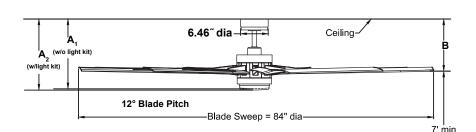
Αı В  $A_2$ 16.33" 16.64 12.20" Fan w/ 6" downrod Fan w/12" downrod 22.33" 22.64" 18.20" 24.20" Fan w/18" downrod 28.33" 28.64" Fan w/24" downrod 34.33" 34.64" 30.20" Fan w/36" downrod 46.33" 46.64" 42.20" Fan w/48" downrod 58.33" 58.64" 54.20" Fan w/60" downrod 70.33" 70.64" 66.20" Fan w/72" downrod 82.33" 82.64" 78.20"
